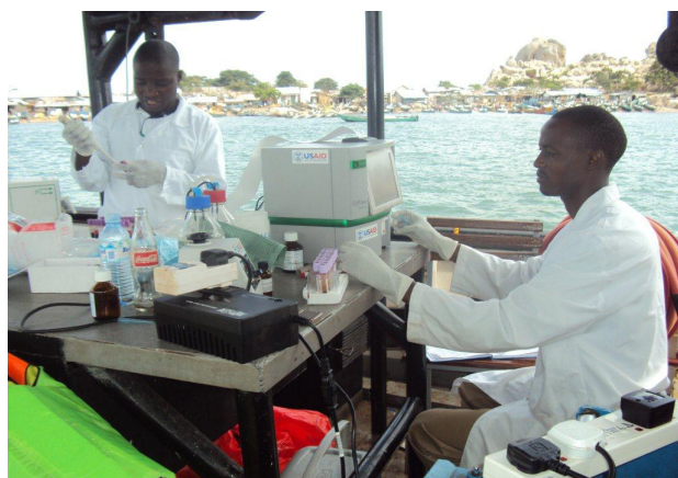
A laboratory unit on a boat. Patients' blood analysis for CD 4 cell count on a Portable CD4 machine in progress.
